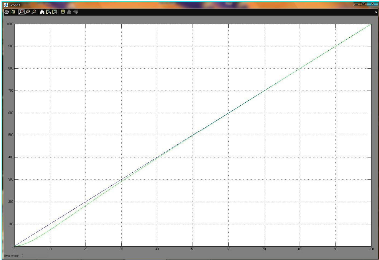
Figure 12 PID Heading Response to a heading RAMP command
